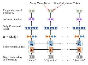
Figure 3: Structure of Head Entity Detection (HED) model.
