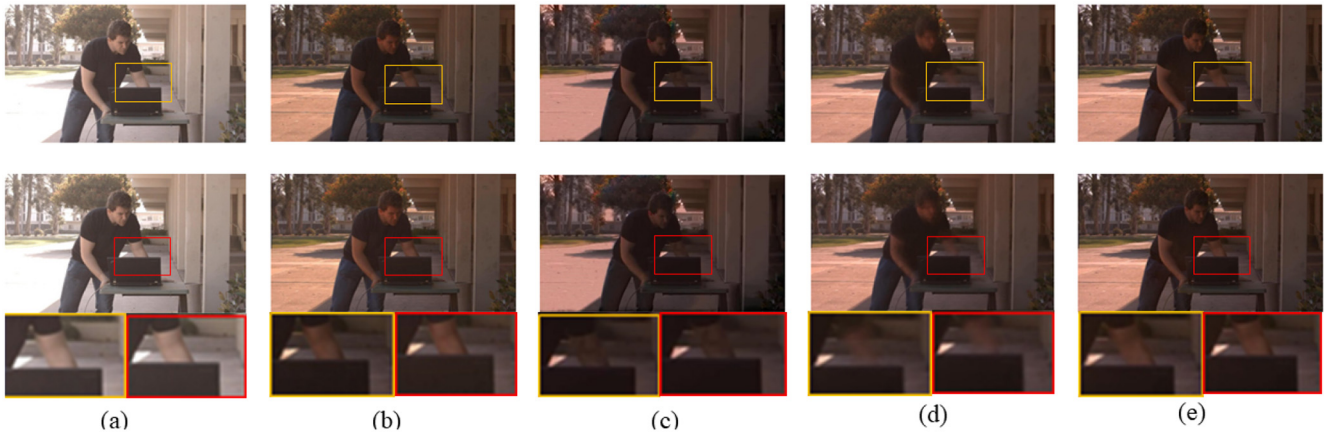
Fig. 15. Experimental results of the checking e-mail video. The top row is the 98th frame, and the bottom row is the 99th frame. (a) Original frames are temporally consistent. (b) After applying the method of HDR tone mapping to the original frames, there is texture variation of the ground in the processed frames (please see corresponding close-up views). (c) There are temporal artifacts in the results of Bonneel et al. [3] (please see the blurring artifacts on the left arm of the man). (d) Phenomenon of blurring artifacts similar to (c) appears in the results of Lang et al. [10]. (e) Temporally consistent results using our proposed TBLS.
