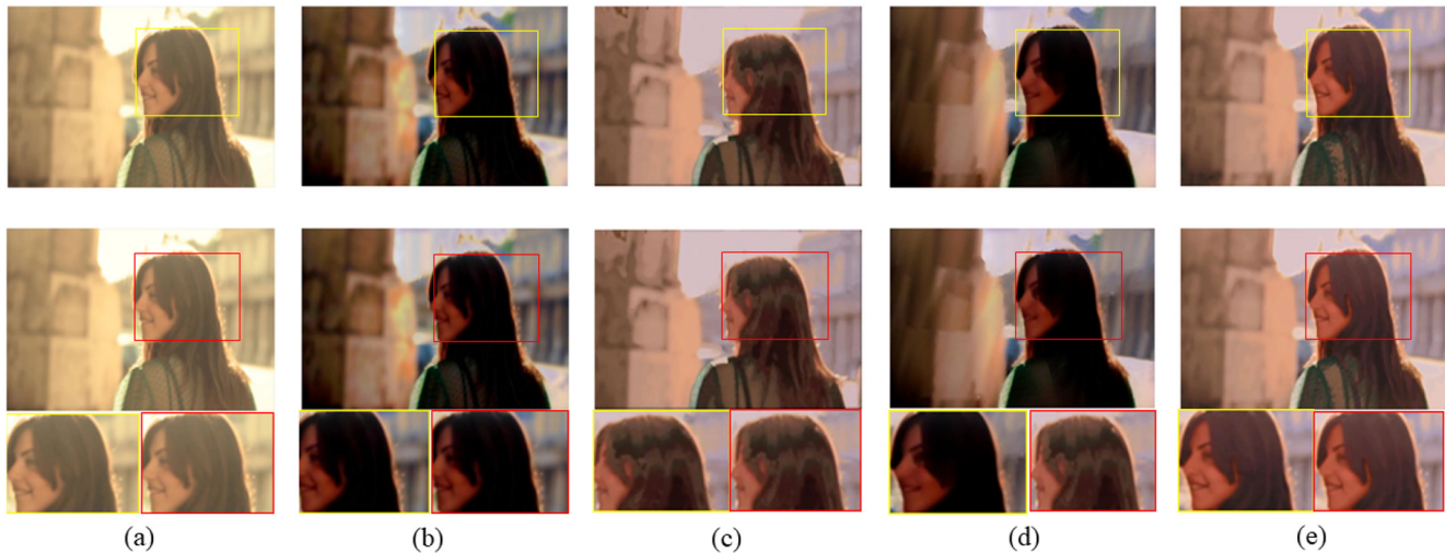
Fig. 14. Experimental results of the lily video. The top row is the 202nd frame, and the bottom row is the 203rd frame. (a) Original frames are temporally consistent. (b) Processed frames are temporally inconsistent, which can be seen from the change of the shining blocks on the wall (please see the fluctuation on the corresponding close-up view). (c) There are temporal artifacts in the results of Bonneel et al. [3] (please see the blurring blocks on the hair of the girl). (d) There are different blurring artifacts in the results of Lang et al. [10]. (e) Results of our proposed TBLS are temporally consistent.
