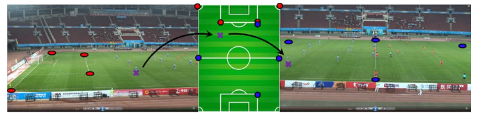
Fig. 7. Use multiview information to automatically find back the lost object. As long as the target is under detection in at least one view, we can use the perspective matrix to obtain its coordinates of bird view. Then, we use another matrix to find its location in another view. We use the original tracking parameters to search in the box and find the target back.
