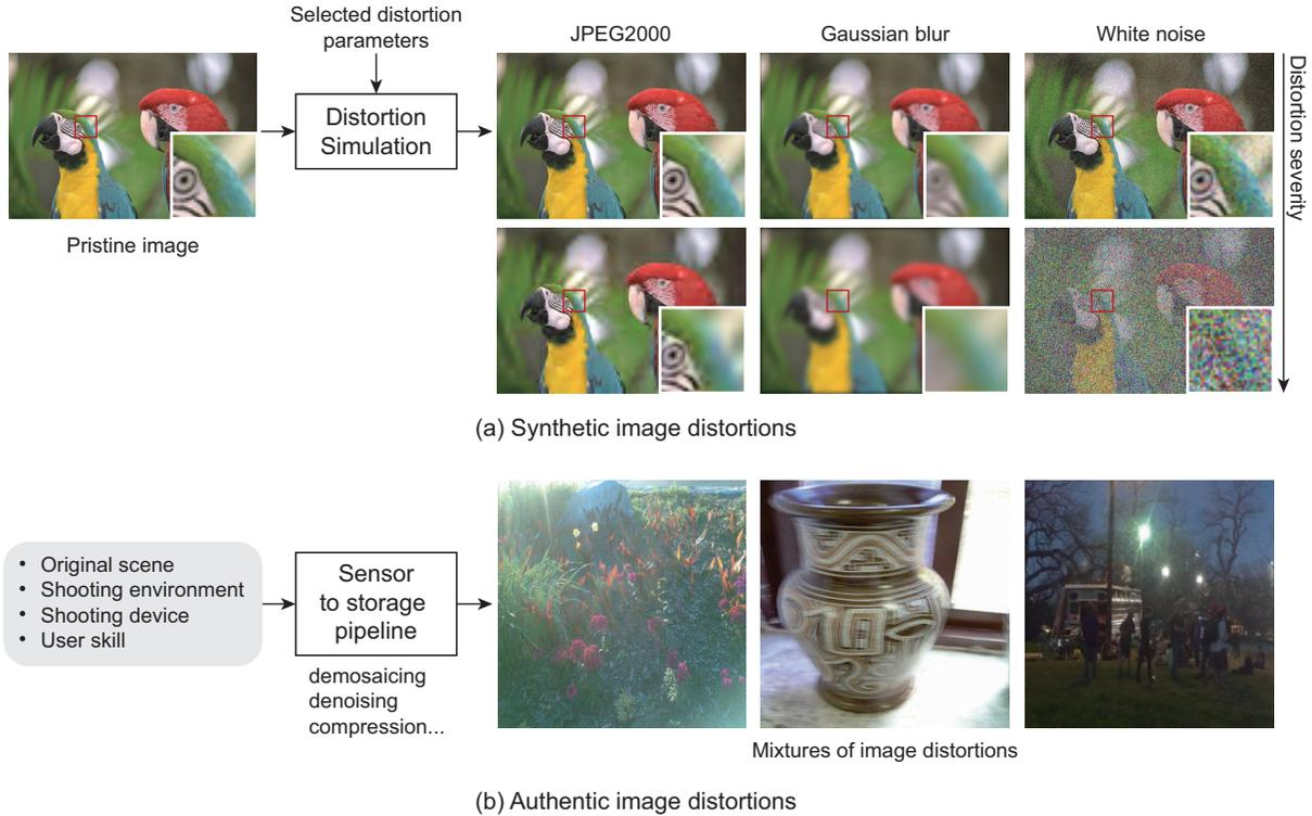
Fig. 5. Synthetic and authentic image distortions found in picture quality databases.
