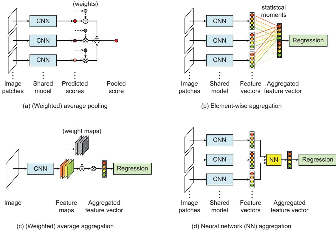
Fig. 4. Examples of aggregation and pooling strategies in CNN-based picture quality prediction models.
