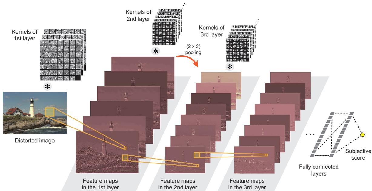
Fig. 1. Example of a CNN structure for no-reference picture quality prediction. The model consists of several convolutional layers followed by a few fully-connected layers. An activation function is applied at each output of the neural network processing flow.
