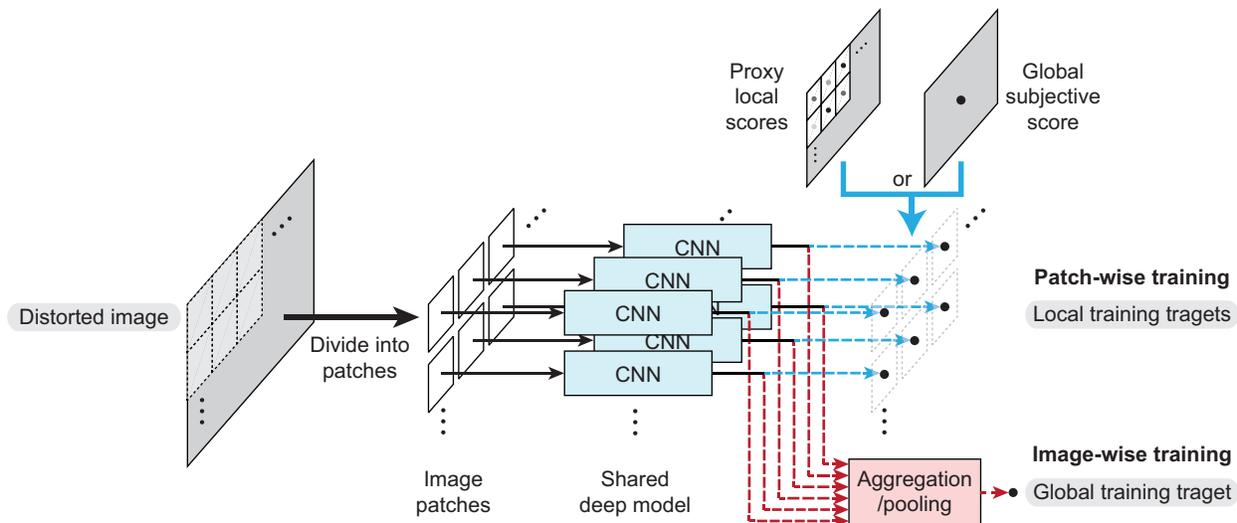
Fig. 3. Patch-wise and image-wise strategies used to train patch-based picture quality prediction models. First, an input image is partitioned into patches, then each is fed into the same CNN model. In patch-wise training, a proxy local score or global subjective score is used as a training target for each input patch. In image-wise training, extracted features or scores are aggregated, then regressed onto a single global subjective score.
