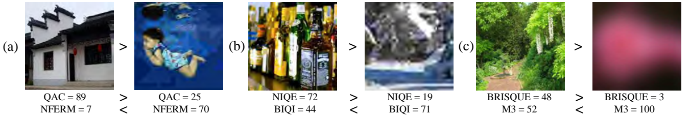
Fig. 5. Sample DIPs from the Exploration database. (a), (b) and (c) show 3 DIPs, where the left images have clearly better quality than the right images. A good model is able to give concordant opinions, whereas a less competitive model tends to perform randomly or provide discordant opinions.
