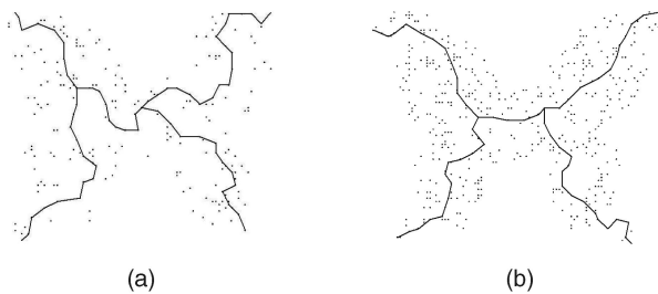
Fig. 14. The skeletons of the butterfly network with different node densities. (a) 250 nodes. (b) 500 nodes.
