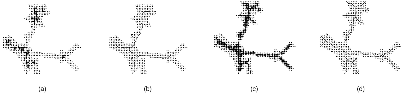
Fig. 12. Comparison on the scenario of JFK airport terminal 5. (a) Medial axis nodes computed by MAP [4]. (b) Medial axis computed by MAP [4]. (c) Skeleton points computed by CASE. (d) Skeleton graph computed by CASE.
