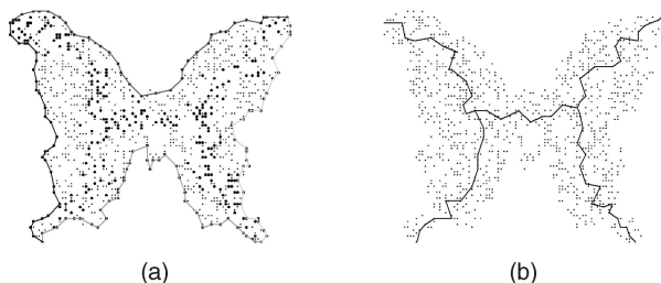
Fig. 16. CASE on the Quasi-UDG in the butterfly network. (a) Skeleton points and segments. (b) Skeleton graph.
