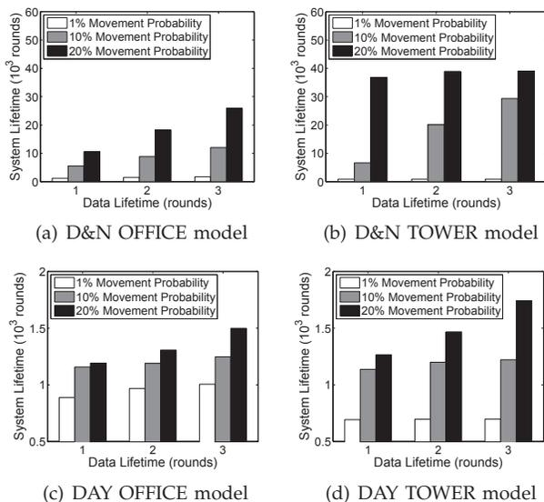
Fig. 11. System lifetime as a function of data lifetime.
