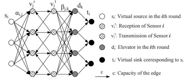
Fig. 4. Graph  $G''(V'', E'')$  and the multi-commodity flow model.
