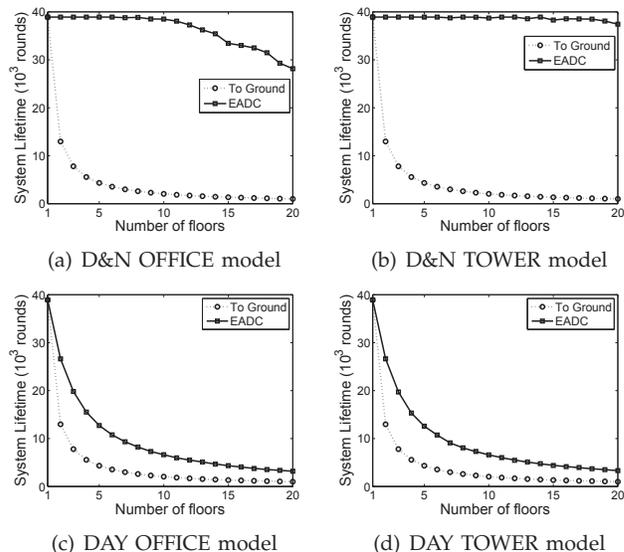
Fig. 7. System lifetime as a function of the number of floors.
