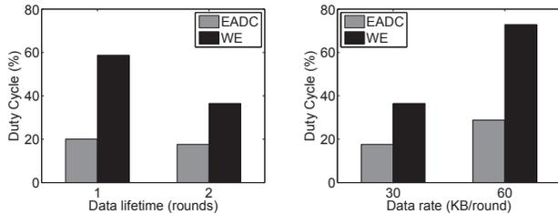
(a) Duty cycle as a function of data lifetime (b) Duty cycle as a function of amount of data
