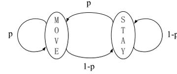
Fig. 6. Elevator movement model used in our simulation.
