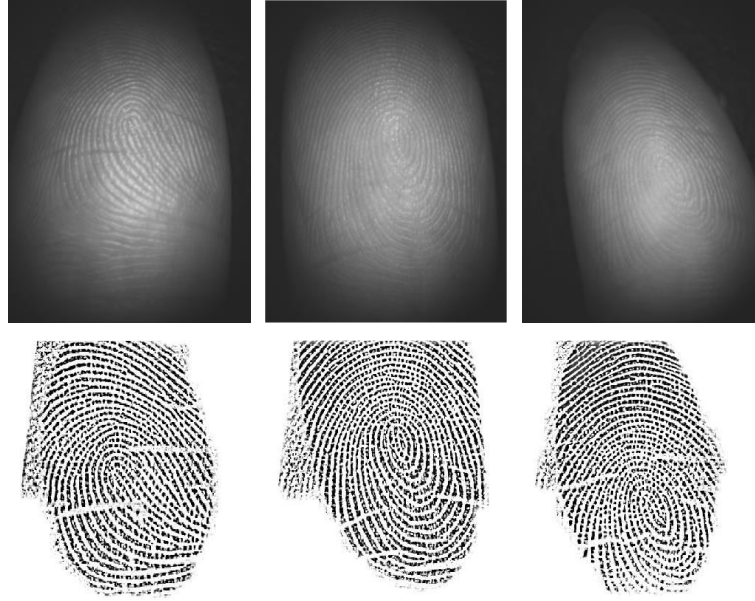
Figure 8: Typical fingerprint samples. top row: contactless fingerprint images, bottom row: corresponding contact-based fingerprint images.
