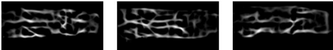
Fig. 2. Enhanced finger vein images to emphasize on vascular features and suppress associated noise. These Gabor filter based enhanced images are respective to ROI in figure 1.
