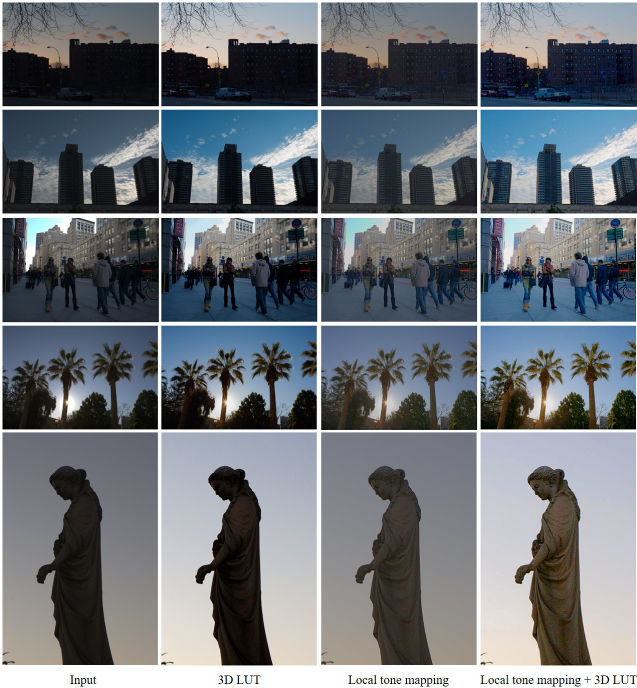
Figure 5: Less satisfied enhancement results of our 3D LUT model. Our model effectively enhances the global color and tone, while the local contrast in the dark areas can be further improved by combining it with some local tone mapping operator. The noise is also amplified in the last example, which can be addressed using some denoising module.
