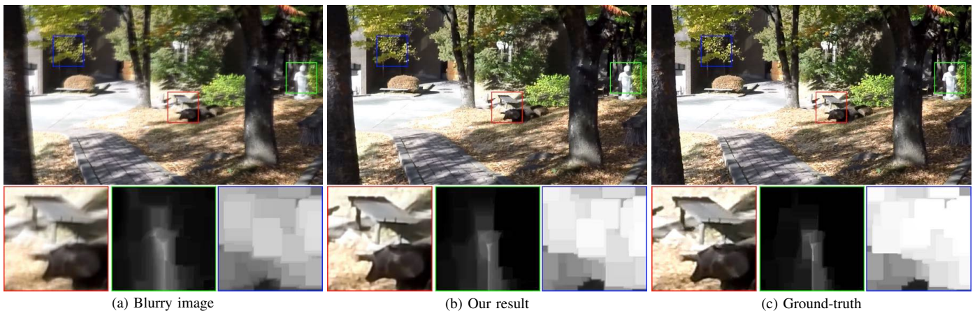
Fig. 1: Deblurring result on a GoPro image [1]. (a) The blurry image; (b) our result; and (c) the Ground-truth image. Red box: zoom-in view of the original local patch. Green box: zoom-in view of the dark channel of its corresponding local patch. Blue box: zoom-in view of the bright channel of its corresponding local patch.
