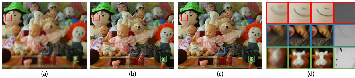
Fig. 2. Our deblurring result. (a) Input blur image with spatially-varying motion blur for objects with different depths. (b) Our result with depth refinement after every 10 iterations of intermediate image updating. (c) Ground-truth image. (d) Close-up view of the three images, with related depths on the right.
