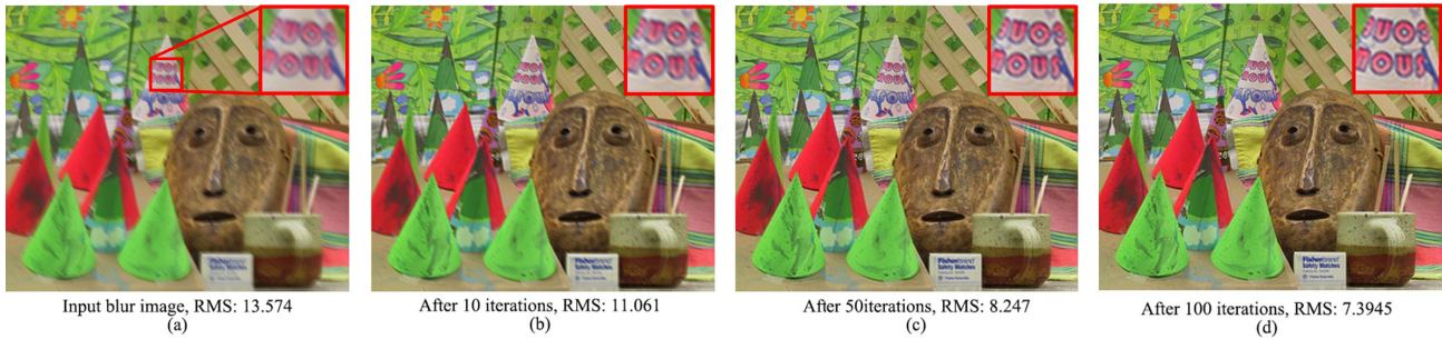
Fig. 13. Decrease in RMS errors with increase in number of iterations. (a) Input blurred image. (b)–(d) Deblurring results after different numbers of iterations.
