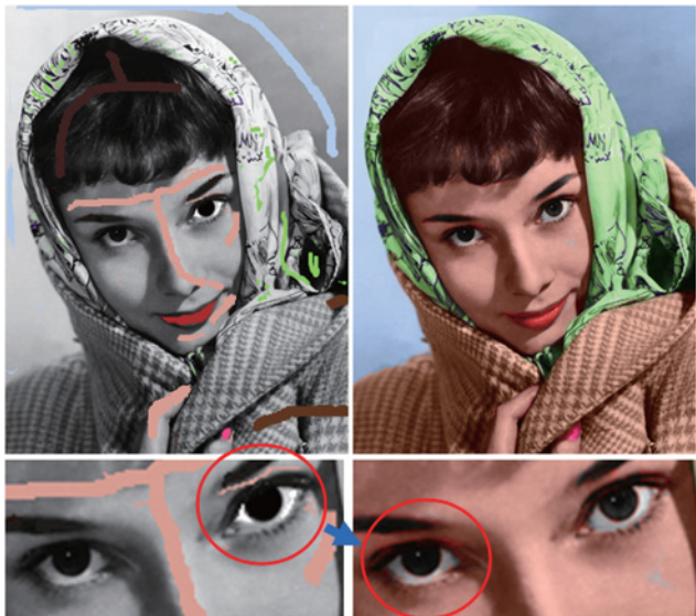
Fig. 12. Colorization using optimization in feature space. (a) Input strokes. (b) Colorization result. Please note that the input colors only existing in the right eye are propagated to the left side.
