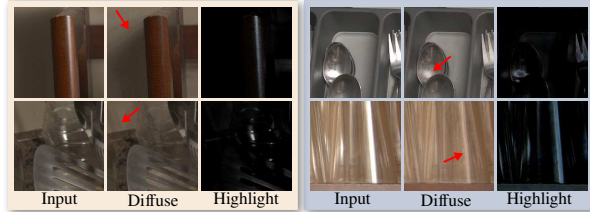
Figure 3. Bad example regions. Left: environment lighting distortion; Right: highlight residual. These pairs need to be removed.
