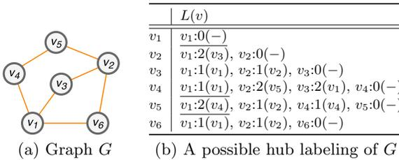
**Figure 2: A hub labeling index fulfilled the cover property (the brackets indicate the predecessors)**
