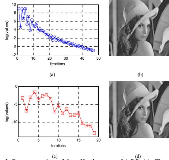
**Fig.2.** Demonstration of the effectiveness of ACC. (a): The difference of objective function between two successive iterations. (c): The difference of ratio  $\gamma$  between two successive iterations. (b): result when  $N_{max}$  is reached (RMSE = 7.05). (d): result of ACC (RMSE = 7.05).
