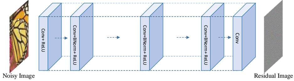
Figure 4. A residual learning based image denoising framework. “Conv” denotes convolution, “ReLU” denotes the rectified linear unit, and “BNorm” denotes batch normalization.
