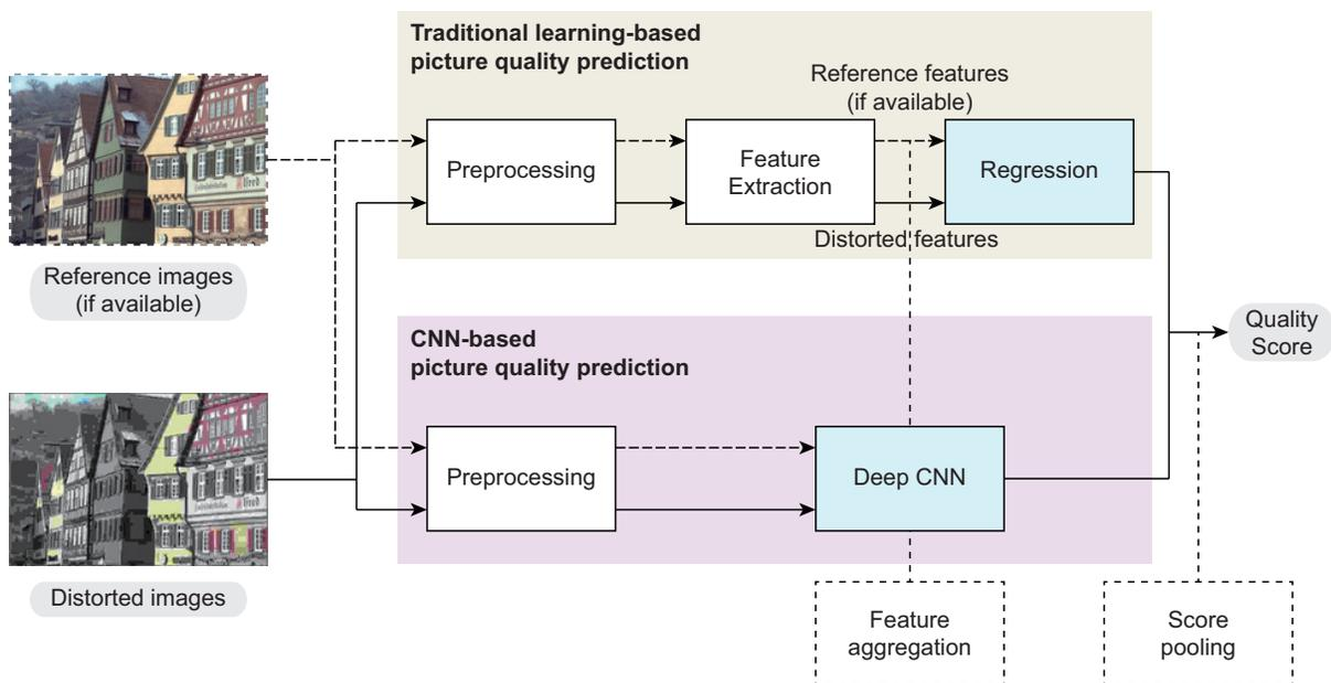
Fig. 2. Flow chart comparisons of traditional learning-based and CNN-based reference and no-reference picture quality models. Blue boxes indicate learning processes.
