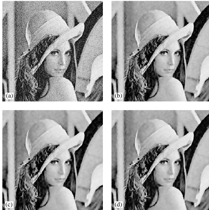
Fig. 5. Denoising results of Lena by wavelet CDF (1,3). (a) Noisy Lena ( \sigma = 30 ). (b) Restored Lena by scheme M1 (SNR = 23.28 dB). (c) Restored Lena by scheme M2 (SNR = 23.71 dB). (d) Restored Lena by scheme M3 (SNR = 24.21 dB).
