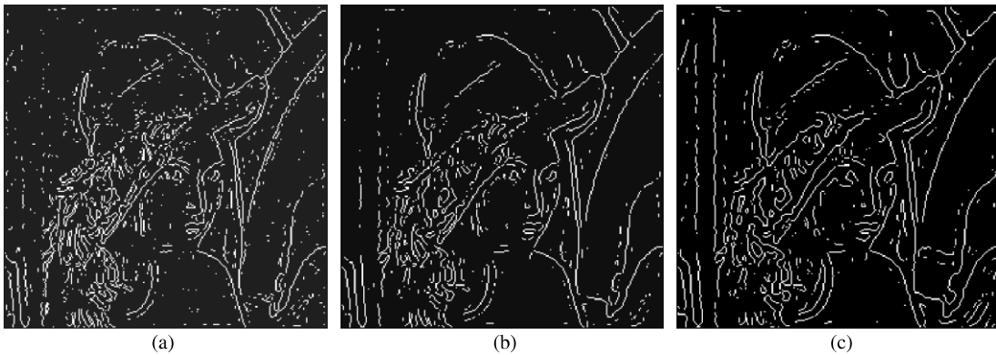
Fig. 14. Edge maps by LOG: (a) \sigma_g = 1.6 , (b) \sigma_g = 2.0 , (c) \sigma_g = 2.4 .
