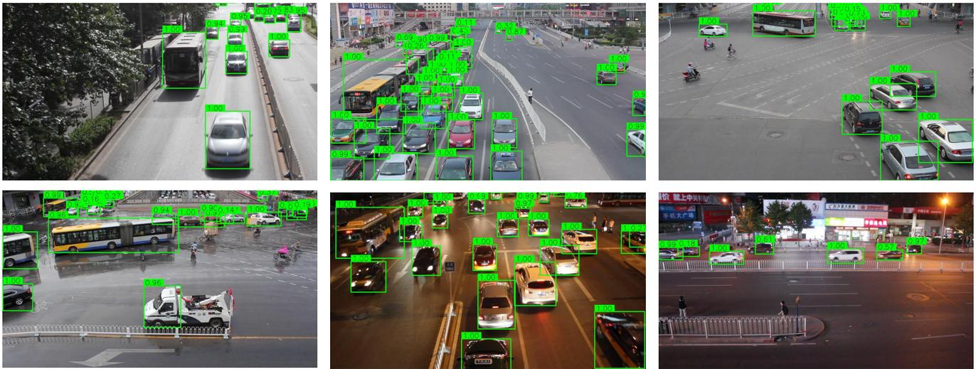
Fig. 8. Examples of detection results in various environmental conditional. A bounding box is plotted if its confidence score is larger than 0.1.
