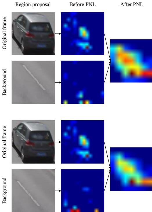
Fig. 10. Feature activations before and after pairwise non-local operation (PNL). For a better visualization, we select only one channel in the feature maps, then map their values to the interval of 0-255, and up-sample the feature channel by bilinear interpolation.
