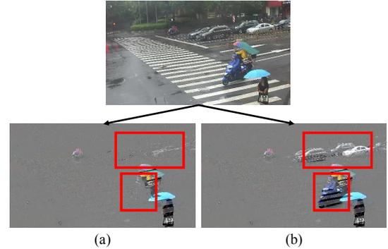
Fig. 3. Foreground frame by (a) OMoGMF [22]; (b) BS-RNN with detection result feedbacks. Static cars and cyclists are preserved as foreground by feedbacks.
