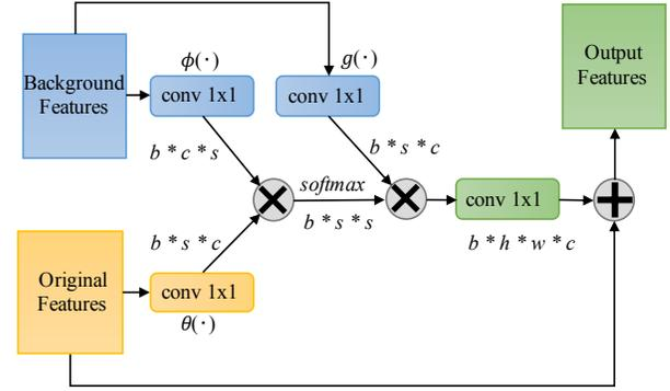
Fig. 6. Details of pairwise non-local operations.  $b * h * w * c$ , namely  $batchsize * height * width * channel$ , indicates the shape of data tensor. For the convenience of matrix operations, we reshape the input tensors to  $b * s * c$ , where  $s = h * w$ , and permute the background tensor to  $b * c * s$ .  $\otimes$  denotes matrix product of two tensors and  $\oplus$  denotes element-wise sum.
