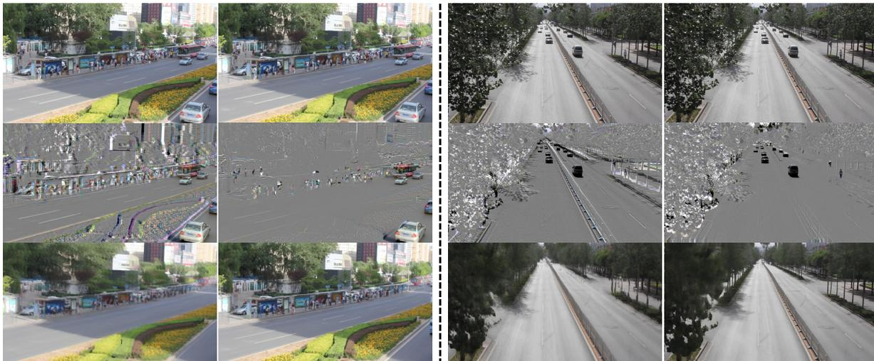
Fig. 7. Explanation of how the image transformation operator deals with the camera vibrations. The left column shows the results of BS-RNN without transformation and the right column shows that of with transformation. The images of each column are original frame, foreground and background from top to bottom.
