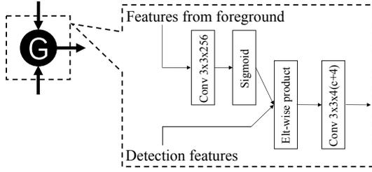
Fig. 5. Details of a gate module. The number of output channel is  $4 \times (c+4)$ .  $c$  denotes class number, the first 4 is anchor number and the second denotes 4 coordinates for localization.
