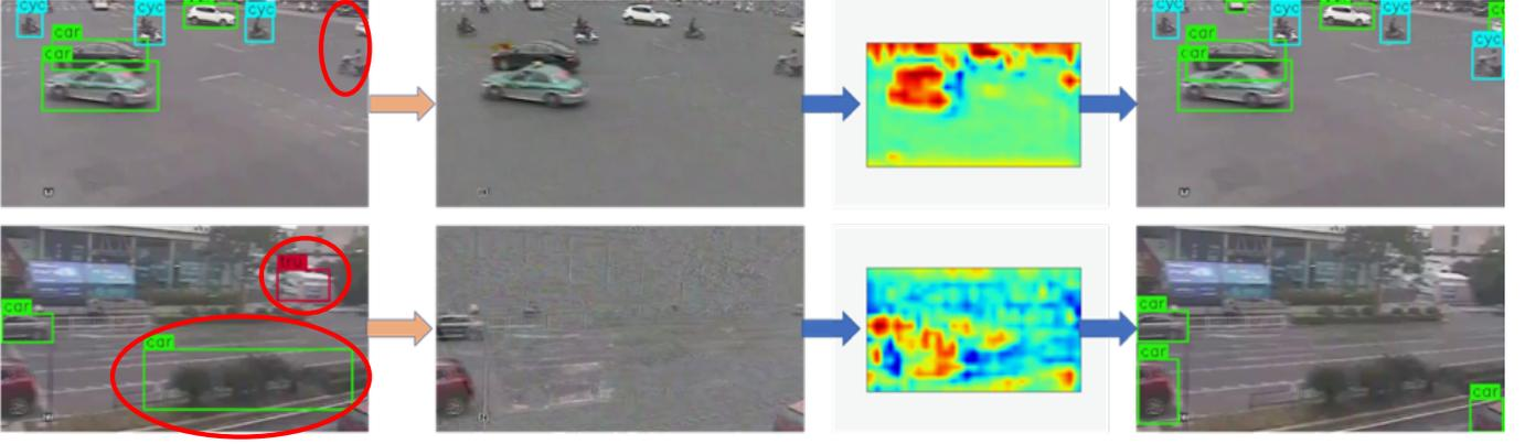
Fig. 4. Explanation of how Foreground Gating stage helps detection. Enhanced by feature masks of the foreground frame, the red circle regions in the left image are finally detected or eliminated. For a simple visualization, we select only one channel in 1/16 (conv4) feature layer and up-sampling it by bilinear interpolation. A bounding box is plotted if its confidence score is larger than 0.3.
