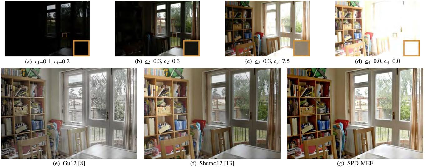
Fig. 2. Making use of color contrast.  $c_k$  is the average signal strength of the  $k$ -th inset patch computed from RGB channels separately.  $c_r$  is the corresponding signal strength by treating RGB channels jointly. Source image sequence by courtesy of Tom Mertens [9].
