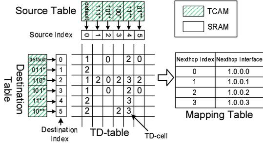
Figure 3: FIST: A forwarding table structure for TwoD-IP
