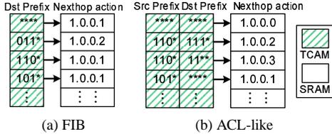
Figure 2: Conventional FIB and ACL-like structures
