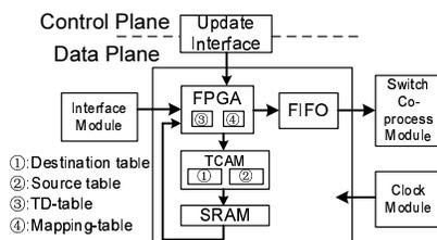
Figure 10: The framework of router design
