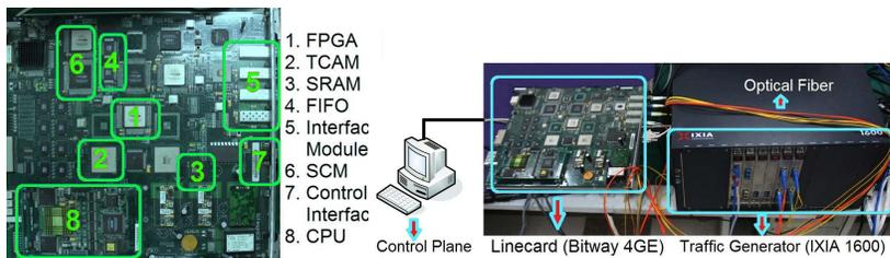
Figure 11: Implementation of FIST on the linecard of Bit-Engine 12004
