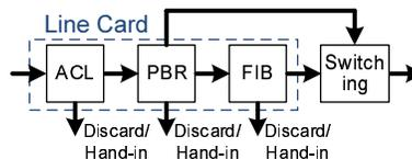
Figure 1: The datapath that packets traverse
