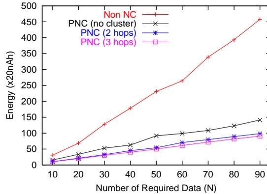
Fig. 7. Energy consumption as a function of  $N$  for different cluster radiuses.
