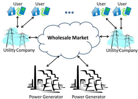
Fig. 1. Advanced metering infrastructure (AMI) system in smart grid.
