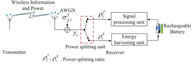
Fig. 2. A block diagram of the receiver model with SWIPT.
