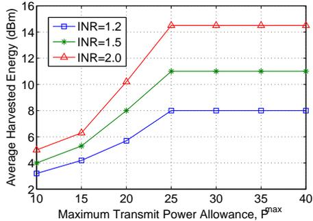
Fig. 6. Average harvested energy (dBm) versus maximum transmit power allowance,  $P^{max}$  for different  $INR$  levels and  $N = 8$ .
