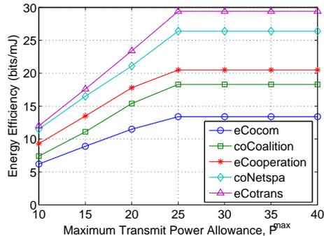
Fig. 8. Energy Efficiency (bits/mJ) versus maximum allowed transmit power for different cooperative schemes.
