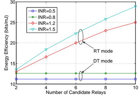
Fig. 5. Energy Efficiency (bits/mJ) versus the number of relay nodes for  $INR = 0.5, 0.8, 1.2, 1.5$ , and  $N = 2, 4, 6, 8, 10$ .
