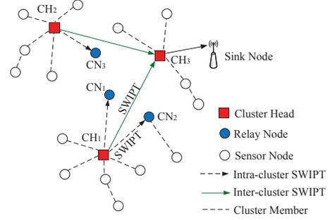
Fig. 1. A clustered wireless sensor network with SWIPT consisting of 3 clusters.
