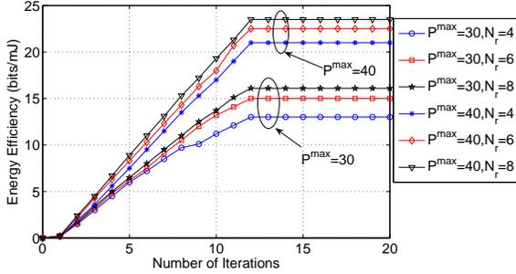
Fig. 4. Energy Efficiency (bits/mJ) versus the number of iterations for  $P^{max} = 30\text{dBm}$  and  $40\text{ dBm}$ , and  $N = 4, 6, 8$ .
