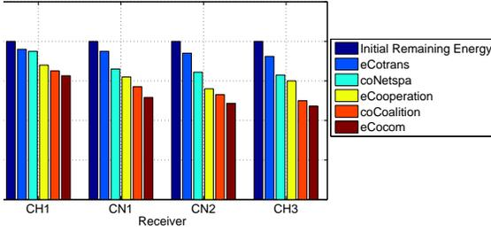
Fig. 9. Remaining energy in the battery versus receivers for different cooperative schemes.
