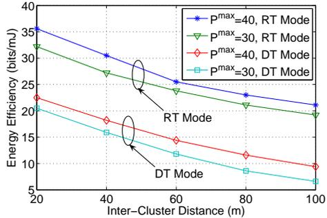
Fig. 7. Energy Efficiency (bits/mJ) versus the inter-cluster distance for  $N = 8$  and  $P^{max} = 30$ dBm, 40dBm.
