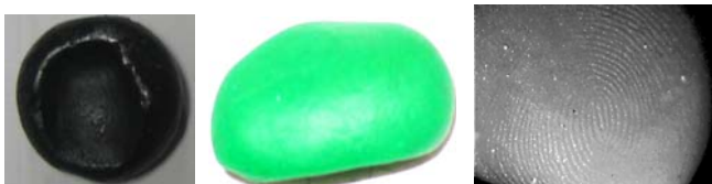
Figure 6: Mold, Play-doh artificial finger and artificial fingerprint.
