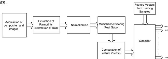
**Figure 1:** Block diagram of experimental setup.
