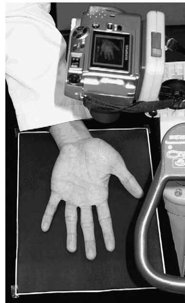
Fig. 2. Acquisition of a typical hand image using digital camera, with our simple setup.
