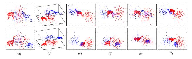
Figure S-3: Examples of matching results by different methods for the occlusion+outlier test. Top row: horse. Bottom row: dinosaur. (a) Before matching (front view); (b) before matching (side view); (c) ours; (d) RPM; (e) CPD; and (f) MG.
