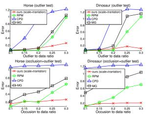
Figure S-2: Average matching errors over 100 random trails by different methods for the 2 categories of tests.
