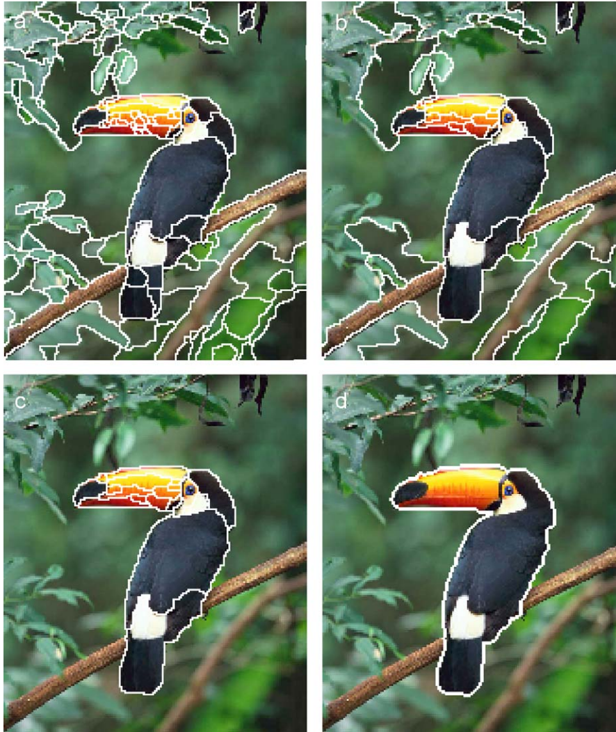
Fig. 2. Region merging process: (a) the first stage (1st round); (b) the second stage (1st round); (c) the first stage (2nd round); and (d) the merging results.
