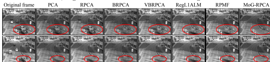
Figure 5. From left to right: original video frames, background extracted by PCA, RPCA, BRPCA, VBRPCA, RegL1ALM, RPMF and MoG-RPCA. The foreground areas are demarcated for easy comparison.
