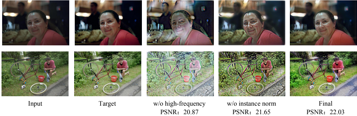
Figure 3. Ablation study toward the model structures on the photo retouching task. The images in the third column are generated without the refinement modules of the high-frequency components, while the images in the fourth column are generated by removing the instance norm layer when translating the low-frequency component. The PSNRs are the average of 500 test images under the specific setting.
