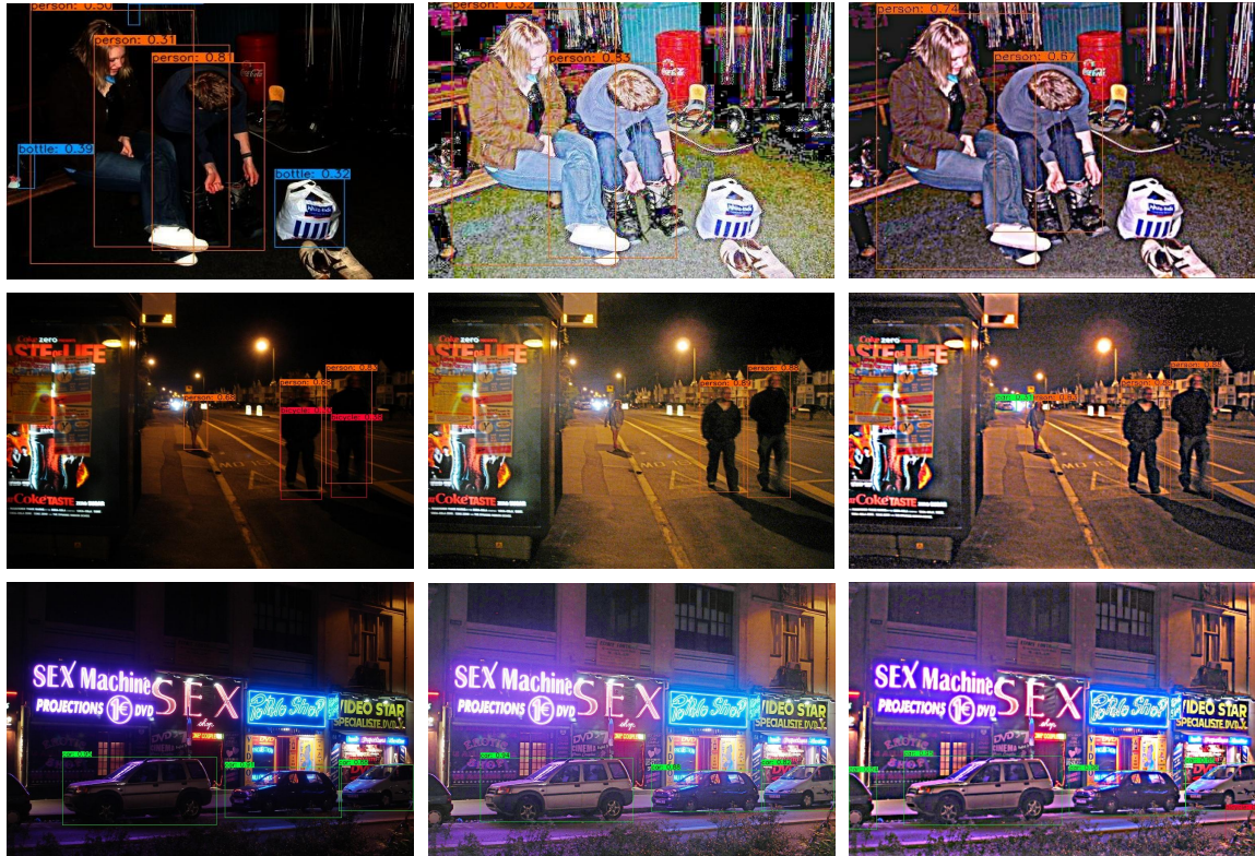
Figure 3: Detection results of different methods on synthetic VOC_Dark_test images (top row), real-world ExDark_test low-light images (bottom two rows). From left to right: YOLOv3 II, ZeroDCE + YOLOv3 I and our IA-YOLO. The proposed method learns to make the image brighter with more details, which results in better detection performance with fewer missed and wrong detections.
