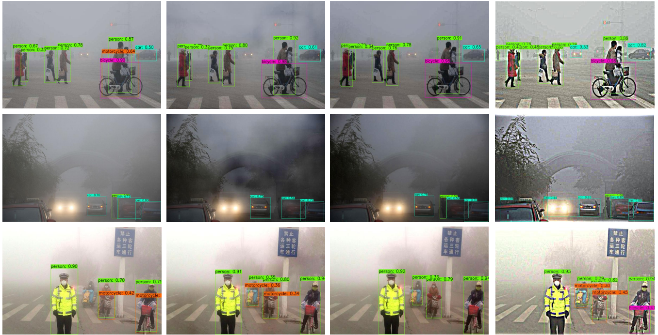
Figure 7: Detection results by different methods on real-world RTTS foggy images. From left to right: YOLOv3 II, GirdDehaze + YOLOv3 I, MSBDN + YOLOv3 I and our IA-YOLO. The proposed method learns to reduce the haze and enhance the image contrast, which leads to better detection performance with fewer missed and wrong detections.
