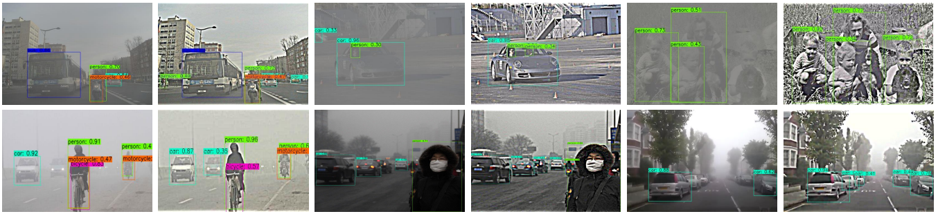
Figure 3: Detection results of YOLOv3 II (columns 1, 3 and 5) and our IA-YOLO (columns 2, 4 and 6) on synthetic VOC_Foggy_test images (top row) and real-world RTTS foggy images (bottom row). The proposed method learns to reduce the haze and sharpen image edge, which has better detection performance with fewer missed and wrong detections.
