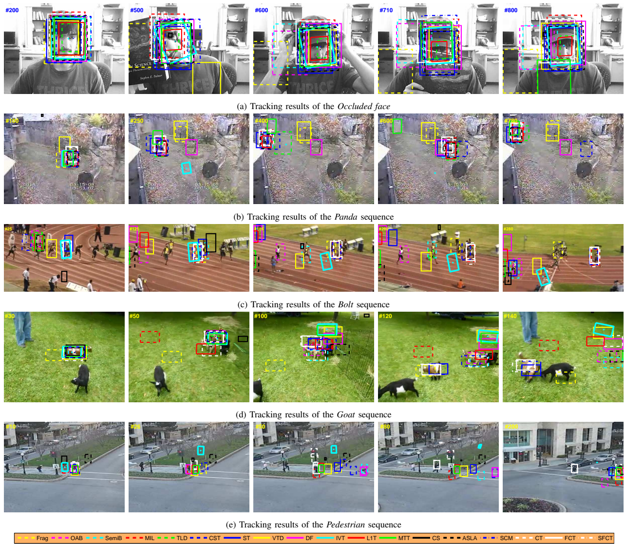
Fig. 9: Screenshots of some sample tracking results when there are severe occlusion and pose variations.
