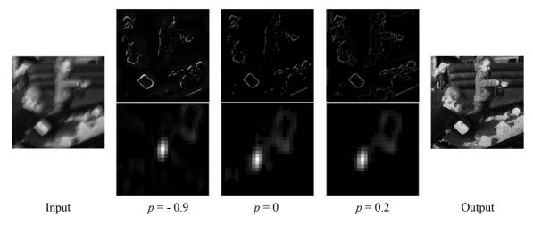
Figure S1: Illustration of intermediate kernel estimation with learned *p* values. The above row provides the gradient maps and the bottom row shows the corresponding estimated kernels.
