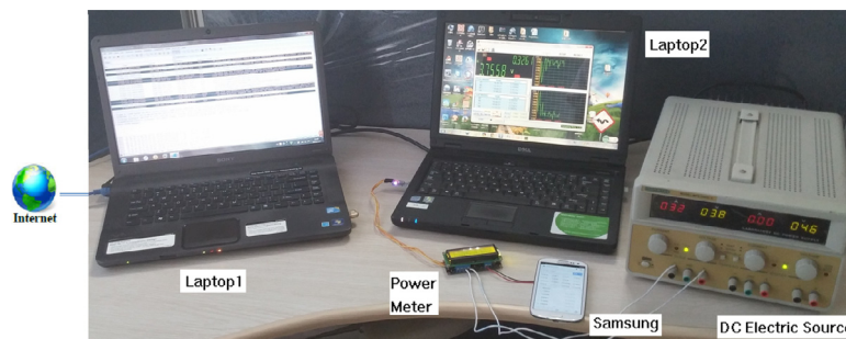
Fig. C.8. The test bed for energy measurement.
