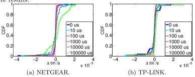
Fig. 8. The CDF of the difference between packet IDTs computed by the DAG card capture and send timestamps reported by OMware ( $\rho = 0$  and  $\lambda = 40$  bytes).
