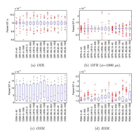
**Fig. 5.** The box-and-whisker plots of packet IDTs using different methods ( $\alpha = 1$  ms, NETGEAR router).
