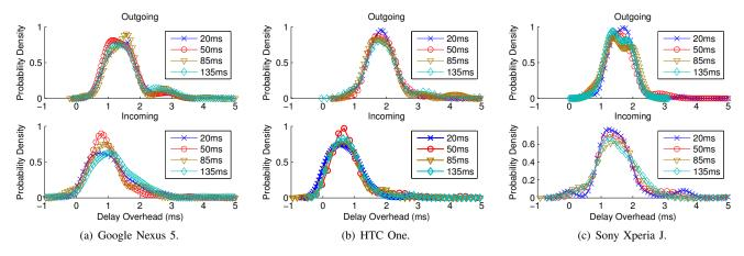
Fig. 7: PDF plots of the delay overhead asymmetry (Inet ping).
