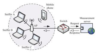
Fig. 2: The testbed setup where the packet sniffers, mobile phone, and wireless AP are placed within a distance of 0.5m.
