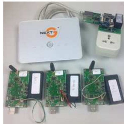
Fig. 5: The Sensor System. Here we present our enhanced Imote2 node and 3 TelosB temperature sensors.
