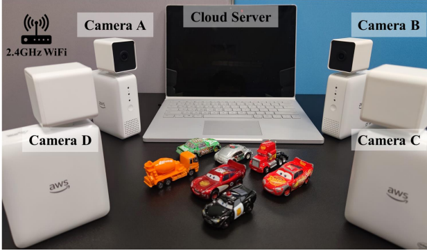
Fig. 4: The schematic of FEVA-supported Multi-view Vehicles 3D Reconstruction system implementation.
